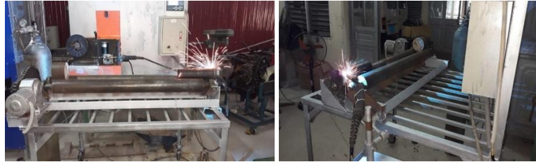
Figure 3. The designed and manufactured welding equipment
