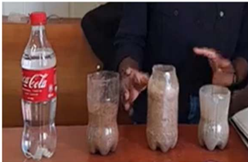
Figure 2: Testing for water infiltration capacity of different types of soils in grade 8
